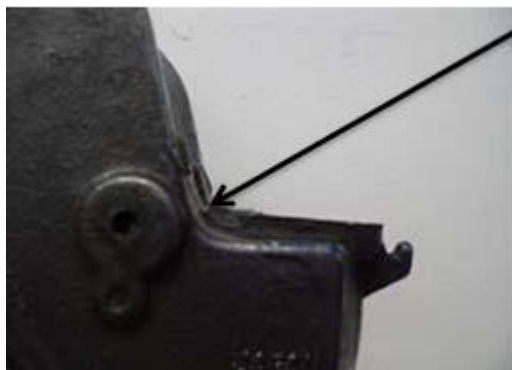
Photo 3: Steering bracket with the turning stop removed
