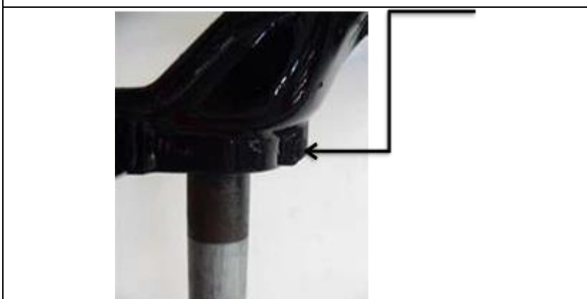
Photo 2: Steering bracket with centre turning lug removed
